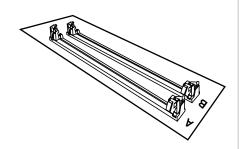
The order in which the slots are used when installing the SIMMs depends on the number of SIMMs added. Refer to the table below.
