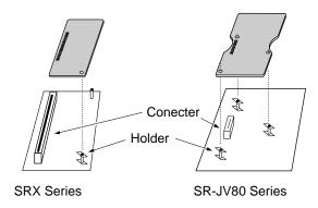
Use the Installation Tool supplied with the Wave Expansion Board to turn the holders in the LOCK direction, so the board will be fastened in place.
